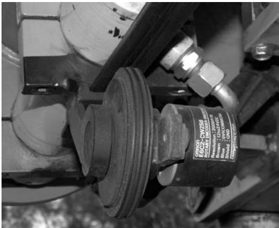
Fig.2 High speed encoder mounted on the mobile arm
